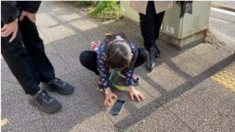
Measuring the slope by MaPiece with the smartphone placed on the ground.
